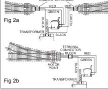
Wire up the point motor (or point motors) as shown in Fig 2a and 2b above. Hornby lever switches are designed to plug together in any number, so you can gather all your switches in a neat bank with minimum wiring (all switches share a common wire to the controller).
